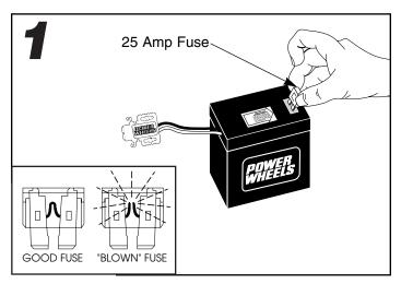
If you are charging the battery for the first time, insert a 25 amp fuse into the battery.
